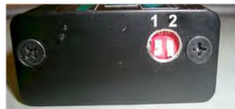
Figure 3 DIP switches and advance curve selection.
